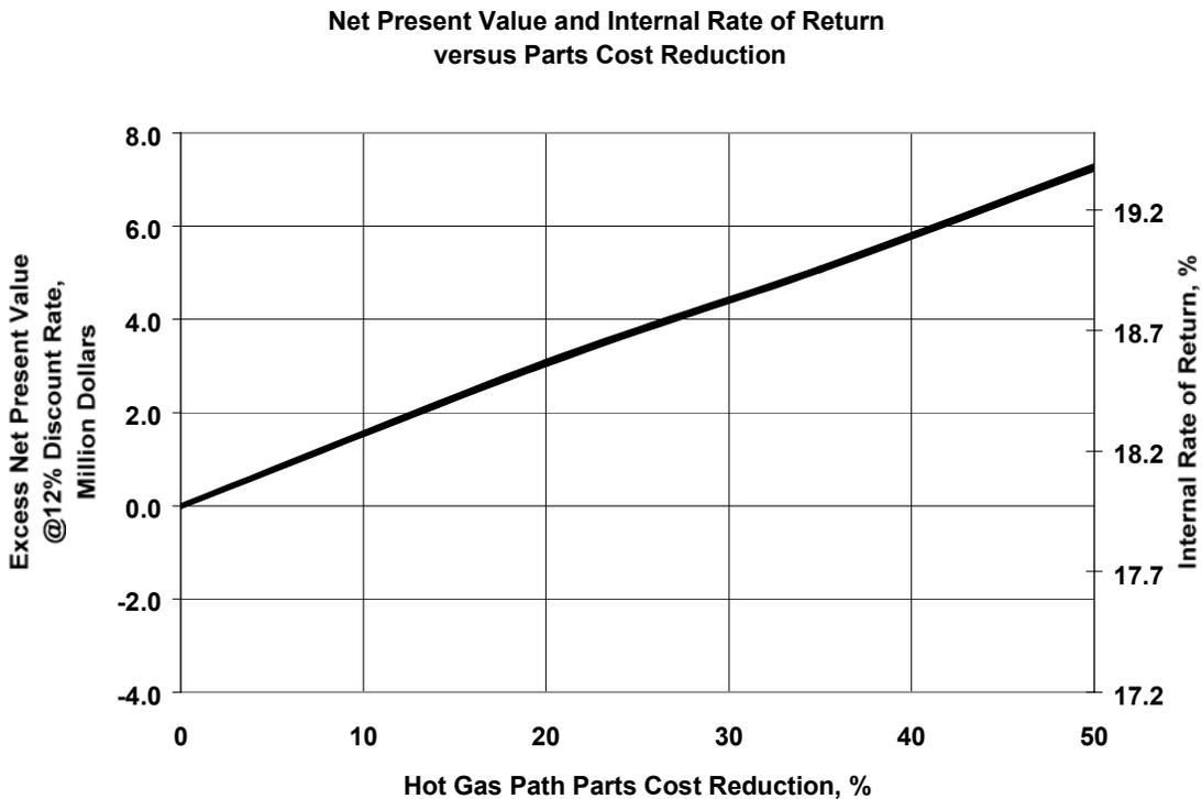
Figure 10- Plant Profitability Sensitive to Reduction in Hot Gas Path Parts Cost
